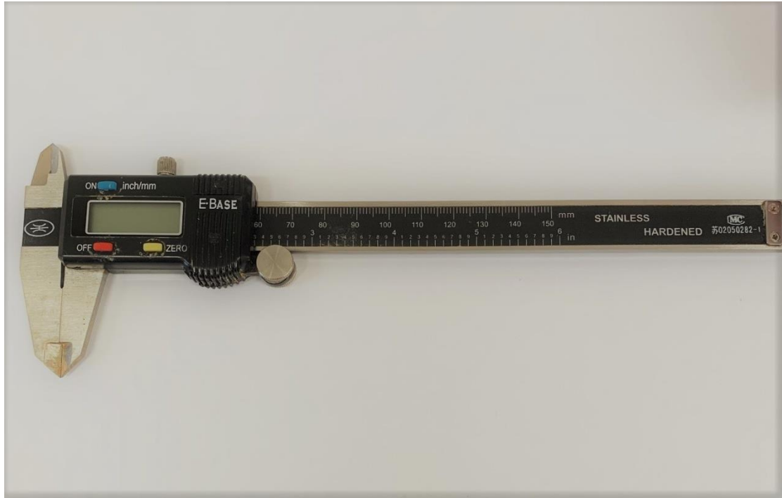
Figure 5: A picture of the digital caliper used in the measurements
