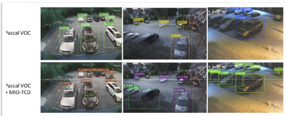
Figure 67: The enhanced SSD-Mobilenet Detector implemented at the edge of our system has a significantly improved detection performance (Ruimin Ke - Yifan Zhuang- Ziyuan Pu and Yinhai Wang, 2020)
