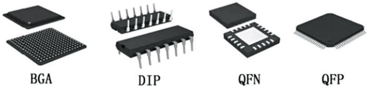
Figure 5: Some IC packaging types
