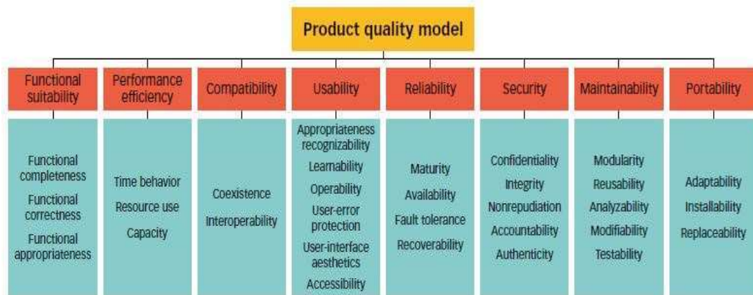
Fig. 3. Eight (8) Characteristics of Software Product Quality Model and System Quality in Use Model
