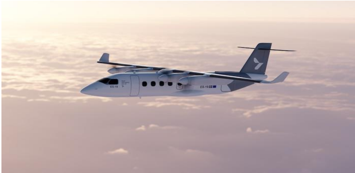
Figure 12 : Above is the electric aircraft ES-19. It is a 19-seater electric plane designed to enhance the economic viability of Air Transport services to remote areas. Heart Aerospace based at Sæve Airport in Gothenburg; Sweden is planning to have its ES-19 operating by 2025.
