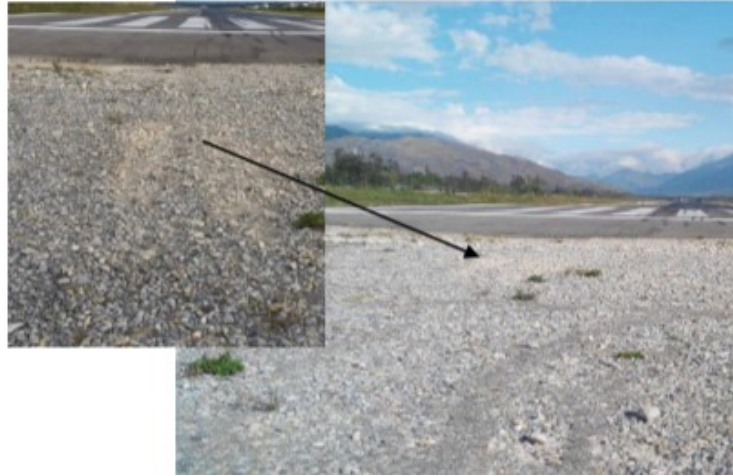
Figure 4.32. Touchdown Mark on The Surface before The Runway (KNKT 2015)
