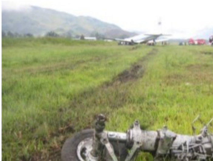
Figure 4.25. BAe ATP Landing Gear Detached (KNKT 2013)
