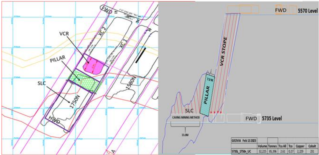
Figure 4: Typical VCR Ore Body and Developments Section
