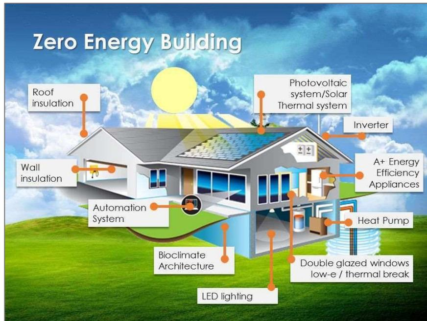
**Pic. 3.4:** A building model reflecting the elements of the conceptual Zero Energy building that makes it a green building. (Ref. 3.2)
