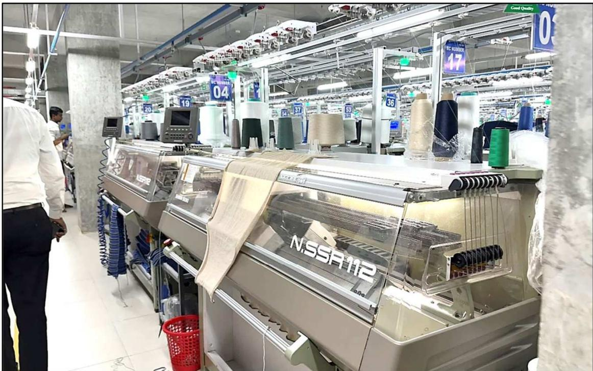
*Pic. 5.4.6 & 5.4.7: Pic of automatic fabric knitting jacquard machine in the factory (Ref:ss)*
